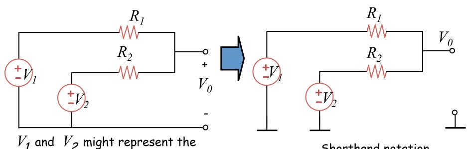
$V_1$  and  $V_2$  might represent the outputs of two sensors, for e.g.
