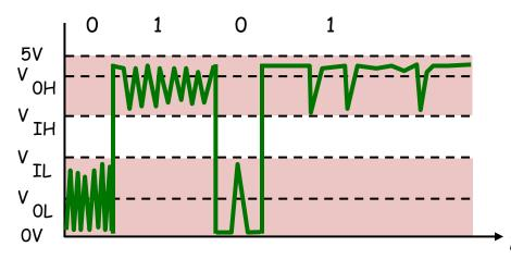
Digital systems follow static discipline: if inputs to the digital system meet valid input thresholds, then the system quarantees its outputs will meet valid output thresholds.
