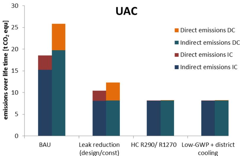
Figure 11: Life time CO<sub>2</sub> emissions in unitary split air conditioning for the business as usual and several emission reduction options in industrialised (IC) and developing countries (DC). An average value has been applied for IC and DC as there are significant differences within those country groups.
