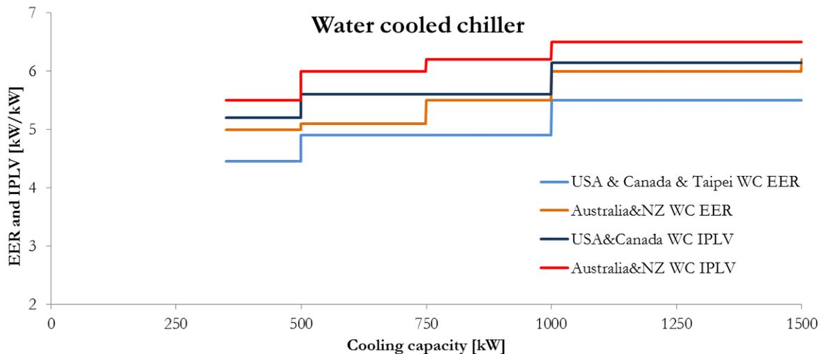
Figure 32: MEPS EER and IPLV requirements for AirC (A) and WC (B) chillers.
