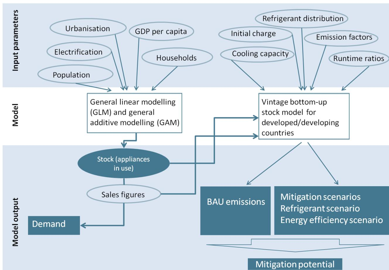
Figure 7: Modelling framework to derive future demand, emission scenarios and mitigation potential
