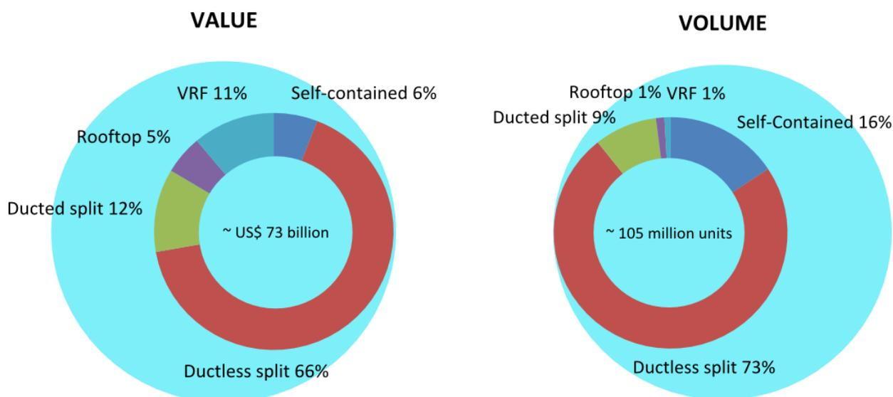
Figure 12: Global demand for residential and commercial UAC systems, divided by appliance system types (2012). (A) shows demand by value in USD and (B) shows the volume in units
