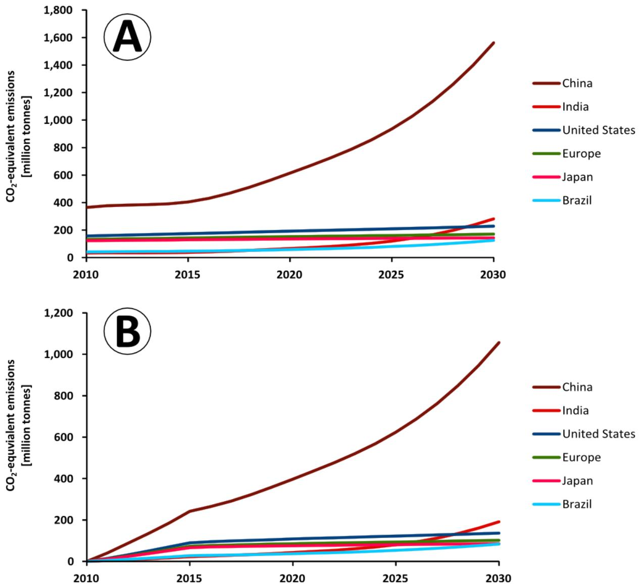
Figure 19: Projected total (direct and indirect) emissions from residential split air conditioners for the top-6 countries as calculated by a vintage bottom-up stock model (A). Key determining factors are stock and sales figures. The upper graph (A) shows the BAU scenario, while the bottom graph (B) shows the mitigation potential.
