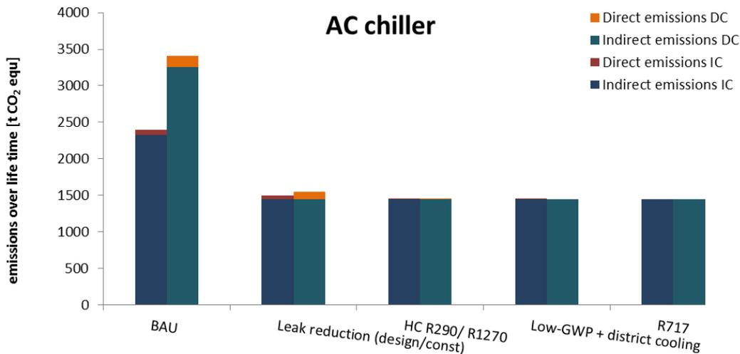
Figure 33: CO<sub>2</sub> emissions over lifetime in AC chillers in developing countries (DC) and industrialised countries (IC) . An average value has been applied for IC and DC as there are significant differences within those country groups.
