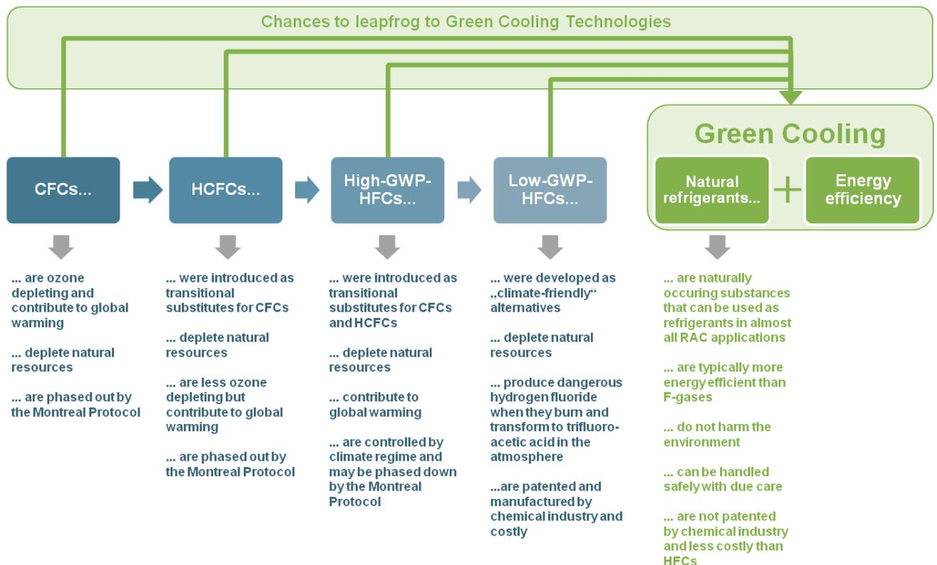
Figure 2: Leapfrogging to green cooling technologies
