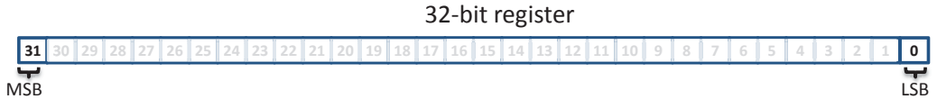
Figure 1.7: Bit numbering for an AXI bus register. The LSB is isolated by the mask 0x0000 0001 , and the MSB is isolated by the mask 0x8000 0000 .
