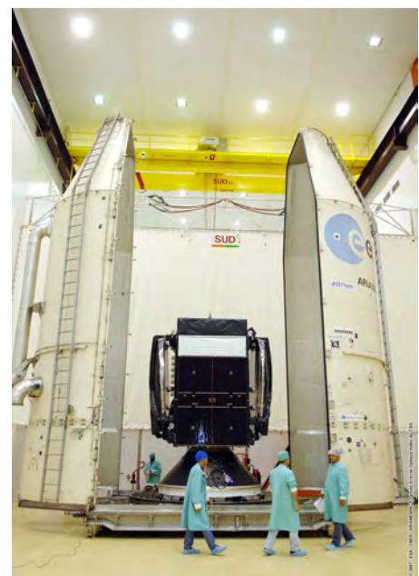
Figure 6.3.4.a – The CCU3 and CCU2 payload containers
