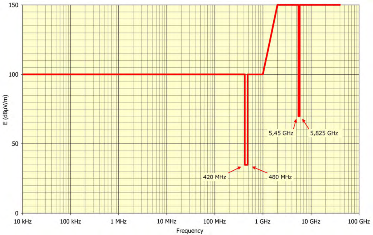
Figure 4.2.5.a – Spurious radiations acceptable to launch vehicle Narrow-band electrical field measured 1.0 m below the separation plane (free space)
