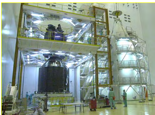
Picture 5.3.4.a – SYLDA 5 Internal carrying structure
