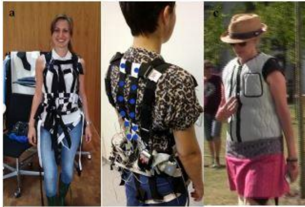
Figure 6. The vibrotactile vest: adjustable harness (a) front and (b) back and (c) outer shell and skirt-apron 27
