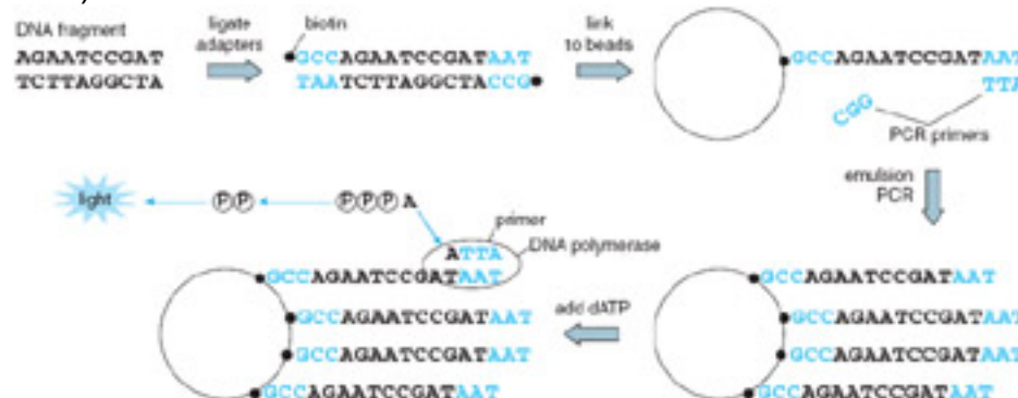
Figure 8.13: Sequencing DNA by the 454 (pyrosequencing) method: adapters are ligated to DNA fragments, immobilized on beads, and amplified by PCR. Solutions of single nucleotides are added and light resulting from an enzymatic reaction involving the pyrophosphate cleaved from the nucleotide when it is added to the DNA chain is detected as evidence that a particular nucleotide was incorporated. Reactions can be done on 1.6 million beads in parallel
