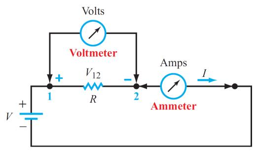
The **ammeter** is the standard instrument used to measure the current flowing between two points in a circuit. To measure I in the circuit above, we insert the ammeter into the current path.
