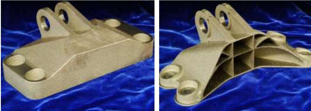
Figure 5: Titanium aircraft bracket produced using (left) conventional manufacturing and (right) additive manufacturing enabling the incorporation of internal cavities that reduce weight while meeting the load requirements (Image ©2016 General Electric Company).
