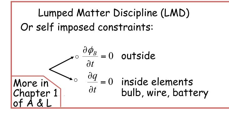
Connecting using ideal wires lumped elements that obey LMD to form an assembly results in the lumped circuit abstraction
