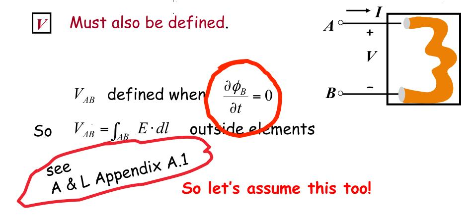
Also, signal speeds of interest should be way lower than speed of light
