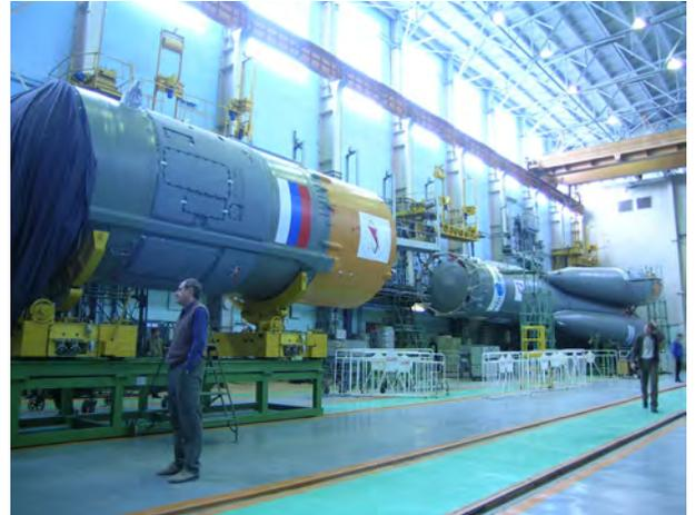
The third stage of the Soyuz 2-1b is powered by the RD-0124 engine.
