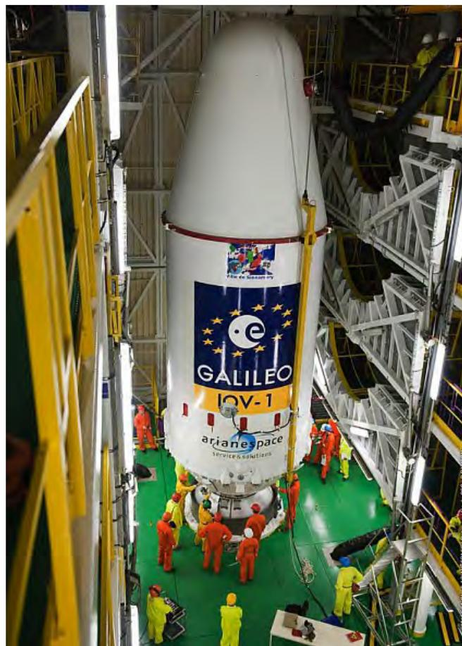
Figure 6.2.3.2.2c – Upper composite hoisting on Launch Vehicle
