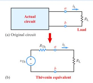
A circuit can be represented in terms of a Thévenin equivalent comprised of a voltage source  $v_{Th}$  in series with a resistance  $R_{Th}$ .
