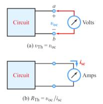
The Thévenin voltage is equal to the open-circuit voltage and Thévenin resistance is equal to the ratio of  $v_{oc}$  to  $i_{sc}$ , where  $i_{sc}$  is the short-circuit current between the output terminals.
